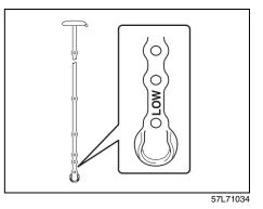
Check that there is washer fluid in the tank by looking at the washer fluid level gauge which is attached to the cap of the washer fluid tank. If the fluid level is near "LOW" mark, refill it.
